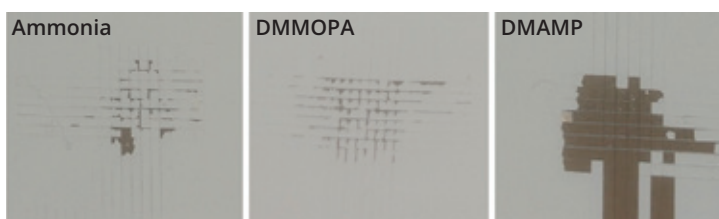
FIGURE 2 » Cross-hatch adhesion of paints neutralized with various amine neutralizers and dried for 7 days.
